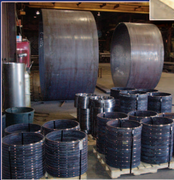
Welded Rings with machined circumferential weld bevels
